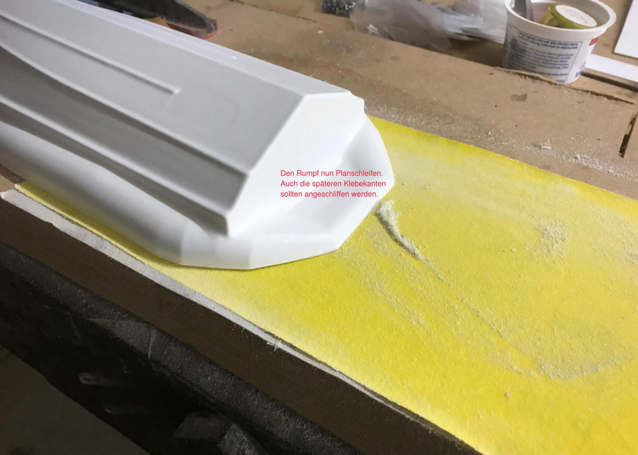
A white, multi-faceted decorative molding piece is being sanded on a yellow surface. The molding has a complex, geometric shape with several flat surfaces and sharp edges. The yellow surface appears to be a workbench or a piece of material being prepared. In the background, there is a white container with some text on it, possibly containing sandpaper or a cleaning agent. The overall scene is a workshop or a DIY project area.
